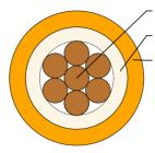
Plain copper conductor NBR modified PVC insulation NBR modified PVC sheath
